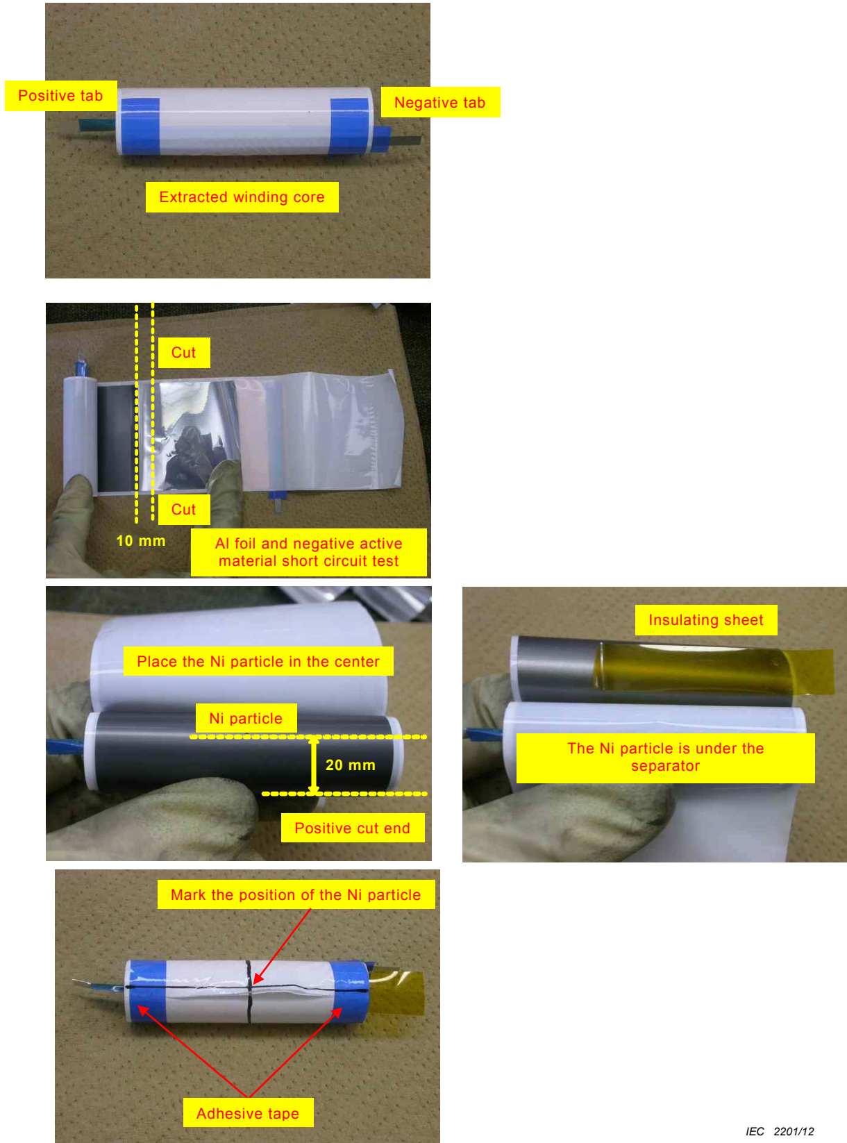
Figure A.5 – Disassembly of cylindrical cell
